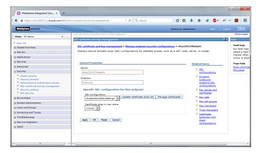
Under SSL configurations, select the configured SSL from the drop-down list.
