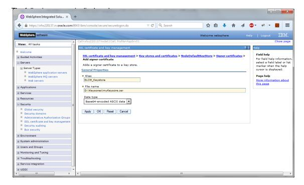
The extracted certificate of the second server has to be imported to the key-store and truststore of first server. This has to be done using the same local path where the extract certificate was generated for the first server.
