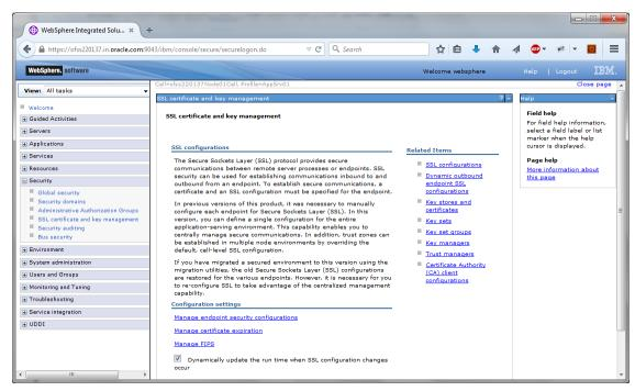
1. Expand 'Security > SSL certificate and key management' and click 'Manage endpoint security configurations'.
